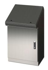
Saginaw desk console, NEMA 3R/4/4X/12/13, 46 x 25 x 19in (HxWxD), freestanding, 304 stainless steel, #4 brush finish, single-door, 3-point keylocking flush swing handle.
