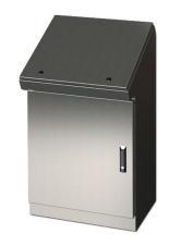
Saginaw desk console, NEMA 3R/4/4X/12/13, 46 x 25 x 19in (HxWxD), freestanding, dual access, 316L stainless steel, #4 brush finish, single-door, 3-point keylocking flush swing handle.
