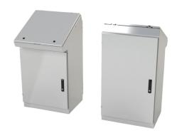
Saginaw desk console, NEMA 3R/4/12/13, 46 x 25 x 19in (HxWxD), freestanding, dual access, carbon steel, ANSI 61 gray, powder coat finish, single-door, 3-point keylocking flush swing handle.
