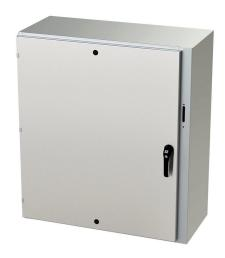
Saginaw Enviroline series disconnect enclosure, NEMA 3R/4/4X/12/13, right flange, 42 x 37 x 16in (HxWxD), wall mount, 316L stainless steel, #4 brush finish, single-door, 3-point padlocking handle, purchase subpanel separately.
