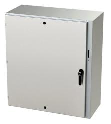
Saginaw Enviroline series disconnect enclosure, NEMA 3R/4/4X/12/13, right flange, 42 x 37 x 16in (HxWxD), wall mount, 316L stainless steel, #4 brush finish, single-door, 3-point padlocking handle, purchase subpanel separately.
