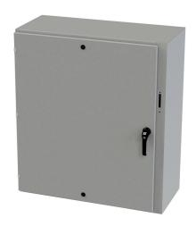
Saginaw Enviroline series disconnect enclosure, NEMA 3R/4/12/13, right flange, 42 x 37 x 16in (HxWxD), wall mount, carbon steel, ANSI 61 gray, powder coat finish, single-door, 3-point padlocking handle, purchase subpanel separately.
