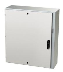
Saginaw Enviroline series disconnect enclosure, NEMA 3R/4/4X/12/13, right flange, 42 x 37 x 12in (HxWxD), wall mount, 304 stainless steel, #4 brush finish, single-door, 3-point padlocking handle, purchase subpanel separately.
