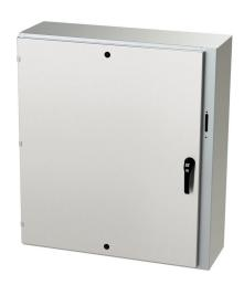
Saginaw Enviroline series disconnect enclosure, NEMA 3R/4/4X/12/13, right flange, 42 x 37 x 12in (HxWxD), wall mount, 316L stainless steel, #4 brush finish, single-door, 3-point padlocking handle, purchase subpanel separately.
