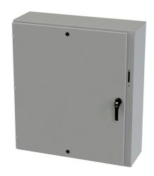
Saginaw Enviroline series disconnect enclosure, NEMA 3R/4/12/13, right flange, 42 x 37 x 12in (HxWxD), wall mount, carbon steel, ANSI 61 gray, powder coat finish, single-door, 3-point padlocking handle, purchase subpanel separately.
