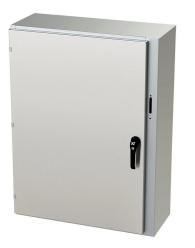
Saginaw Enviroline series disconnect enclosure, NEMA 3R/4/4X/12/13, right flange, 42 x 31 x 12in (HxWxD), wall mount, 316L stainless steel, #4 brush finish, single-door, 3-point padlocking handle, purchase subpanel separately.
