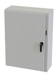
Saginaw Enviroline series disconnect enclosure, NEMA 3R/4/12/13, right flange, 42 x 31 x 12in (HxWxD), wall mount, carbon steel, RAL 7035 light gray, powder coat finish, single-door, 3-point padlocking handle, purchase subpanel separately.
