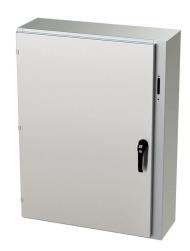
Saginaw Enviroline series disconnect enclosure, NEMA 3R/4/4X/12/13, right flange, 42 x 31 x 10in (HxWxD), wall mount, 304 stainless steel, #4 brush finish, single-door, 3-point padlocking handle, purchase subpanel separately.
