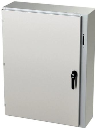
Saginaw Enviroline series disconnect enclosure, NEMA 3R/4/4X/12/13, right flange, 42 x 31 x 10in (HxWxD), wall mount, 316L stainless steel, #4 brush finish, single-door, 3-point padlocking handle, purchase subpanel separately.
