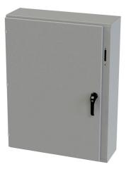
Saginaw Enviroline series disconnect enclosure, NEMA 3R/4/12/13, right flange, 42 x 31 x 10in (HxWxD), wall mount, carbon steel, ANSI 61 gray, powder coat finish, single-door, 3-point padlocking handle, purchase subpanel separately.
