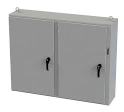
Saginaw disconnect enclosure, NEMA 3R/4/12/13, right flange, 42 x 54 x 12in (HxWxD), freestanding/wall-mount, carbon steel, ANSI 61 gray, powder coat finish, 2-door, 3-point padlocking handle, purchase subpanel separately.
