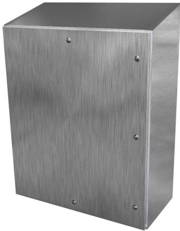
Saginaw sanitary enclosure, slope top, NEMA 3R/4/4X/12, 42 x 36 x 16in (HxWxD), wall mount, 304 stainless steel, #4 brush finish, single-door, 1/4-turn sanitary stainless steel latch.
