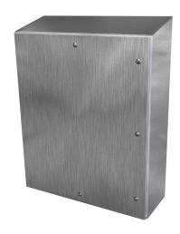
Saginaw sanitary enclosure, slope top, NEMA 3R/4/4X/12,  $42 \times 36 \times 12$ in (HxWxD), wall mount, 304 stainless steel, #4 brush finish, single-door, 1/4-turn sanitary stainless steel latch.
