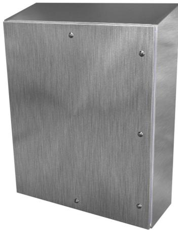
Saginaw sanitary enclosure, slope top, NEMA 3R/4/4X/12, 42 x 36 x 12in (HxWxD), wall mount, 304 stainless steel, #4 brush finish, single-door, 1/4-turn sanitary stainless steel latch.
