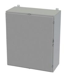
Saginaw enclosure, NEMA 3R/4/12/13, 42 x 36 x 16in (HxWxD), wall mount, carbon steel, ANSI 61 gray, powder coat finish, single-door, plated steel clamps, padlock hasp and staple.
