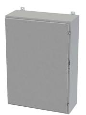
Saginaw enclosure, NEMA 3R/4/12/13, 42 x 30 x 12in (HxWxD), wall mount, carbon steel, ANSI 61 gray, powder coat finish, single-door, plated steel clamps, padlock hasp and staple.
