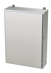
Saginaw enclosure, NEMA 3R/4/4X/12/13, 42 x 30 x 10in (HxWxD), wall mount, 304 stainless steel, #4 brush finish, single-door, stainless steel clamps, padlock hasp and staple.
