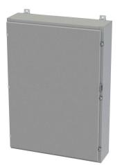
Saginaw enclosure, NEMA 3R/4/12/13, 42 x 30 x 8in (HxWxD), wall mount, carbon steel, ANSI 61 gray, powder coat finish, single-door, plated steel clamps, padlock hasp and staple.
