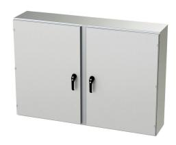
Saginaw Enviroline series enclosure, NEMA 3R/4/4X/12/13, 42 x 60 x 12in (HxWxD), wall mount, 304 stainless steel, #4 brush finish, 2-door, 3-point keylocking/padlocking combo handle.
