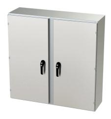
Saginaw Enviroline series enclosure, NEMA 3R/4/4X/12/13, 42 x 42 x 12in (HxWxD), wall mount, 304 stainless steel, #4 brush finish, 2-door, 3-point keylocking/padlocking combo handle.
