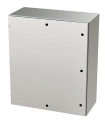
Saginaw Enviroline series enclosure, NEMA 3R/4/4X/12/13, 42 x 36 x 16in (HxWxD), wall mount, 316L stainless steel, #4 brush finish, single-door, 1/4-turn semi-flush latch.
