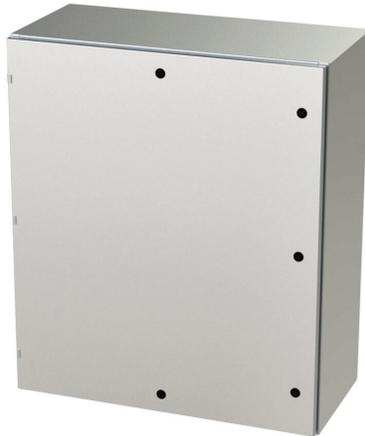
Saginaw Enviroline series enclosure, NEMA 3R/4/4X/12/13, 42 x 36 x 16in (HxWxD), wall mount, 316L stainless steel, #4 brush finish, single-door, 1/4-turn semi-flush latch.
