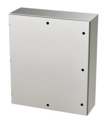
Saginaw Enviroline series enclosure, NEMA 3R/4/4X/12/13,  $42 \times 36 \times 12$ in (HxWxD), wall mount, 304 stainless steel, #4 brush finish, single-door, 1/4-turn semi-flush latch.
