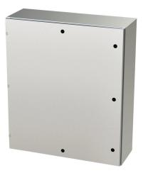
Saginaw Enviroline series enclosure, NEMA 3R/4/4X/12/13,  $42 \times 36 \times 12$ in (HxWxD), wall mount, 316L stainless steel, #4 brush finish, single-door, 1/4-turn semi-flush latch.
