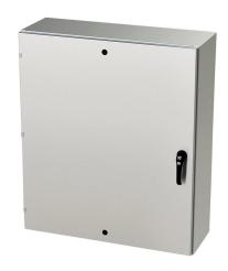
Saginaw Enviroline series enclosure, NEMA 3R/4/4X/12/13, 42 x 36 x 12in (HxWxD), wall mount, 316L stainless steel, #4 brush finish, single-door, 3-point keylocking/padlocking combo handle.
