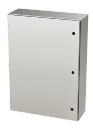
Saginaw Enviroline series enclosure, NEMA 3R/4/4X/12/13,  $42 \times 30 \times 10$  in (HxWxD), wall mount, 304 stainless steel, #4 brush finish, single-door, 1/4-turn semi-flush latch.
