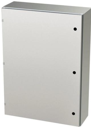
Saginaw Enviroline series enclosure, NEMA 3R/4/4X/12/13, 42 x 30 x 10in (HxWxD), wall mount, 304 stainless steel, #4 brush finish, single-door, 1/4-turn semi-flush latch.
