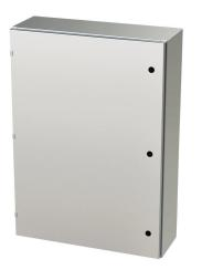
Saginaw Enviroline series enclosure, NEMA 3R/4/4X/12/13,  $42 \times 30 \times 10$ in (HxWxD), wall mount, 316L stainless steel, #4 brush finish, single-door, 1/4-turn semi-flush latch.
