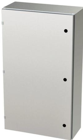
Saginaw Enviroline series enclosure, NEMA 3R/4/4X/12/13, 42 x 24 x 10in (HxWxD), wall mount, 304 stainless steel, #4 brush finish, single-door, 1/4-turn semi-flush latch.
