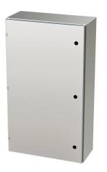
Saginaw Enviroline series enclosure, NEMA 3R/4/4X/12/13,  $42 \times 24 \times 10$ in (HxWxD), wall mount, 316L stainless steel, #4 brush finish, single-door, 1/4-turn semi-flush latch.
