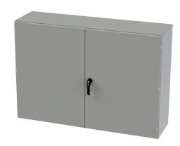
Saginaw enclosure, NEMA 3R/12/13, 42 x 60 x 16in (HxWxD), wall mount, carbon steel, ANSI 61 gray, powder coat finish, doubledoor, 3-point keylocking/padlocking combo handle.
