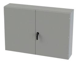
Saginaw enclosure, NEMA 3R/12/13, 42 x 60 x 12in (HxWxD), wall mount, carbon steel, ANSI 61 gray, powder coat finish, double-door, 3-point keylocking/padlocking combo handle.
