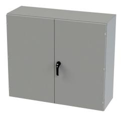
Saginaw enclosure, NEMA 3R/12/13, 42 x 48 x 16in (HxWxD), wall mount, carbon steel, ANSI 61 gray, powder coat finish, double-door, 3-point keylocking/padlocking combo handle.
