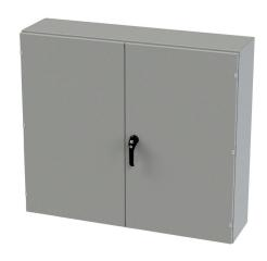
Saginaw enclosure, NEMA 3R/12/13, 42 x 48 x 12in (HxWxD), wall mount, carbon steel, ANSI 61 gray, powder coat finish, doubledoor, 3-point keylocking/padlocking combo handle.
