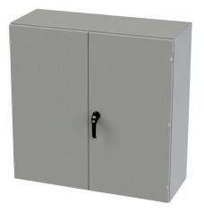
Saginaw enclosure, NEMA 3R/12/13, 42 x 42 x 16in (HxWxD), wall mount, carbon steel, ANSI 61 gray, powder coat finish, double-door, 3-point keylocking/padlocking combo handle.
