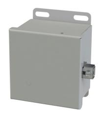
Saginaw enclosure, NEMA 3R/4/12/13,  $4 \times 4 \times 3$ in (HxWxD), wall mount, carbon steel, ANSI 61 gray, powder coat finish, single-door, stainless steel clamps.
