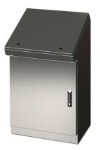
Saginaw desk console, NEMA 3R/12/13/4/4X, 40 x 37 x 16in (HxWxD), freestanding, 304 stainless steel, #4 brush finish, single-door, 3-point keylocking flush swing handle.
