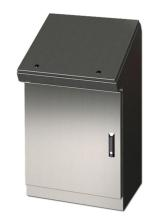
Saginaw desk console, NEMA 3R/12/13, 40 x 37 x 16in (HxWxD), freestanding, 316L stainless steel, #4 brush finish, single-door, 3-point keylocking flush swing handle.
