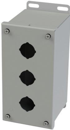
Saginaw pushbutton enclosure, 3 holes, 30mm, NEMA 4/12/13, 8 x 4 x 5in (HxWxD), wall mount, carbon steel, ANSI 61 gray, powder coat finish, screw cover.
