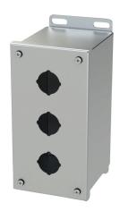
Saginaw pushbutton enclosure, 3 holes, 30mm, NEMA 4/4X/12/13, 8 x 4 x 5in (HxWxD), wall mount, 304 stainless steel, #4 brush finish, screw cover.
