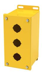
Saginaw pushbutton enclosure, 3 holes, 30mm, NEMA 4/12/13, 8 x 4 x 5in (HxWxD), wall mount, carbon steel, RAL 1018 yellow, powder coat finish, screw cover.
