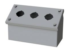
Saginaw pushbutton consolet, 3 holes, 30mm, NEMA 4/12/13, 4 x 8 x 5in (HxWxD), wall mount, carbon steel, ANSI 61 gray, powder coat finish, screw cover.
