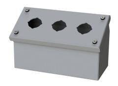
Saginaw pushbutton consolet, 3 holes, 30mm, NEMA 4/12/13,  $4 \times 8 \times 5$  in (HxWxD), wall mount, carbon steel, ANSI 61 gray, powder coat finish, screw cover.
