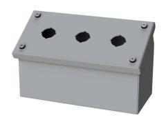
Saginaw pushbutton consolet, 3 holes, 22mm, NEMA 4/12/13, 4  $\times$  8  $\times$  5in (HxWxD), wall mount, carbon steel, ANSI 61 gray, powder coat finish, screw cover.
