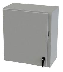
Saginaw Enviroline series disconnect enclosure, NEMA 3R/4/12/13, right flange, 36 x 31 x 16in (HxWxD), wall mount, carbon steel, ANSI 61 gray, powder coat finish, single-door, 2-point padlocking handle, purchase subpanel separately.
