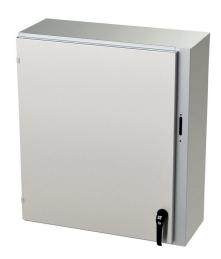
Saginaw Enviroline series disconnect enclosure, NEMA 3R/4/4X/12/13, right flange, 36 x 31 x 12in (HxWxD), wall mount, 304 stainless steel, #4 brush finish, single-door, 2-point padlocking handle, purchase subpanel separately.
