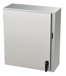
Saginaw Enviroline series disconnect enclosure, NEMA 3R/4/4X/12/13, right flange, 36 x 31 x 12in (HxWxD), wall mount, 316L stainless steel, #4 brush finish, single-door, 2-point padlocking handle, purchase subpanel separately.
