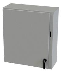
Saginaw Enviroline series disconnect enclosure, NEMA 3R/4/12/13, right flange, 36 x 31 x 12in (HxWxD), wall mount, carbon steel, ANSI 61 gray, powder coat finish, single-door, 2-point padlocking handle, purchase subpanel separately.
