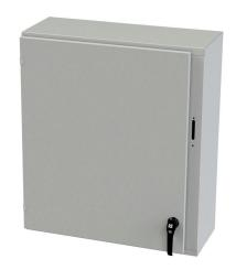
Saginaw Enviroline series disconnect enclosure, NEMA 3R/4/12/13, right flange, 36 x 31 x 12in (HxWxD), wall mount, carbon steel, RAL 7035 light gray, powder coat finish, single-door, 2-point padlocking handle, purchase subpanel separately.
