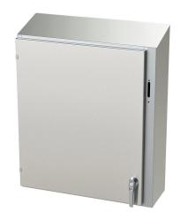
Saginaw Enviroline series disconnect enclosure, slope top, NEMA 3R/4/4X/12/13, right flange, 36 x 31 x 10in (HxWxD), wall mount, 304 stainless steel, #4 brush finish, single-door, 2-point padlocking handle, purchase subpanel separately.
