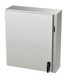
Saginaw Enviroline series disconnect enclosure, NEMA 3R/4/4X/12/13, right flange, 36 x 31 x 10in (HxWxD), wall mount, 304 stainless steel, #4 brush finish, single-door, 2-point padlocking handle, purchase subpanel separately.
